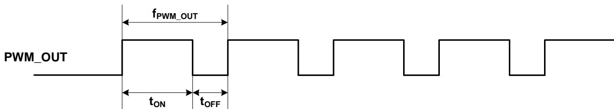
**Note:** The output frequency tolerance of internal frequency divider in CABC is  $\pm 10\%$
